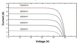
\*Note 1: The specifications are obtained under the standard test conditions: 1000W/m2 solar irradiance, 1.5 Air Mass and cell temperature of 25°C. Measurement uncertainty for all panels is 6%. The actual transactions will be subject to the contracts. These parameters are for reference only and it is not a part of the contracts. The specifications are subject to change without prior notice.
